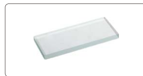
50mm reading scale (check magnification accuracy)
