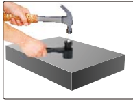
hammer impact to apply test force
