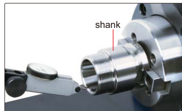
measure radial runout of shank
