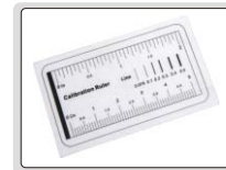
plastic calibration rule (included, graduation 1mm)
