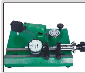
inspect accuracy of dial indicators (range 0-25mm)
