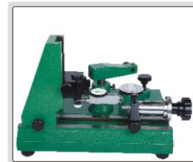
inspect accuracy of test indicators
