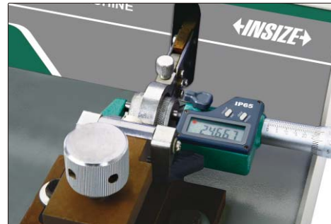
lapping measuring surfaces of outside micrometer
