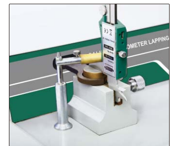
lapping measuring surfaces of caliper lower jaws
