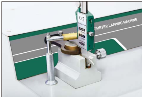
lapping measuring surfaces of caliper lower jaws
