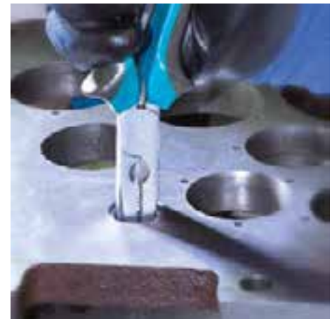
5th operation Breaking of the driving notch with a special cutter
