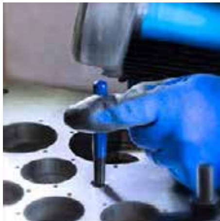
5th operation Breaking of the driving notch with a special cutter
