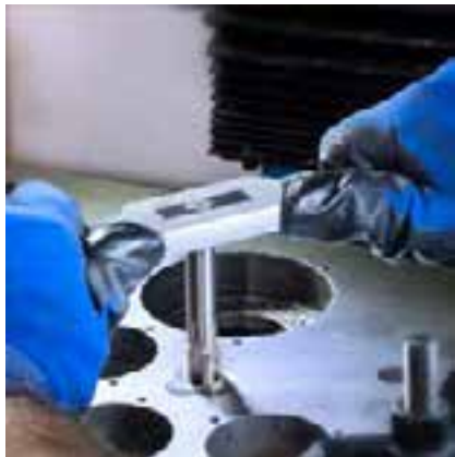
5th operation Breaking of the driving notch with a special cutter
