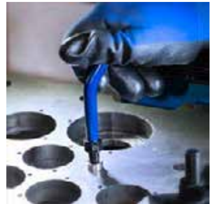
5th operation Breaking of the driving notch with a special cutter
