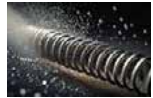
Sandblasting with glass balls (shot peening)
